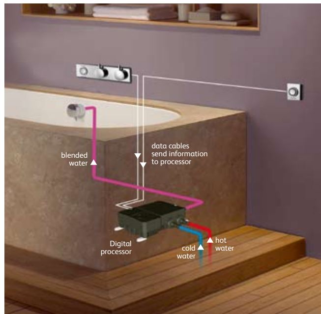
HiQu Bath with overflow filler, remote control, and a high pressure/combination boiler system Digital processor installed under the bath.
